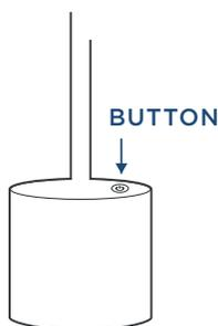
The button located on the base enables you to turn the lamp on and set it to one of the **three brightness levels: 25% - 50% - 100%**. It can easily be charged using the cable and USB charger included in the package. The battery life ranges from 6 to 24 hours per charge based on the brightness.
